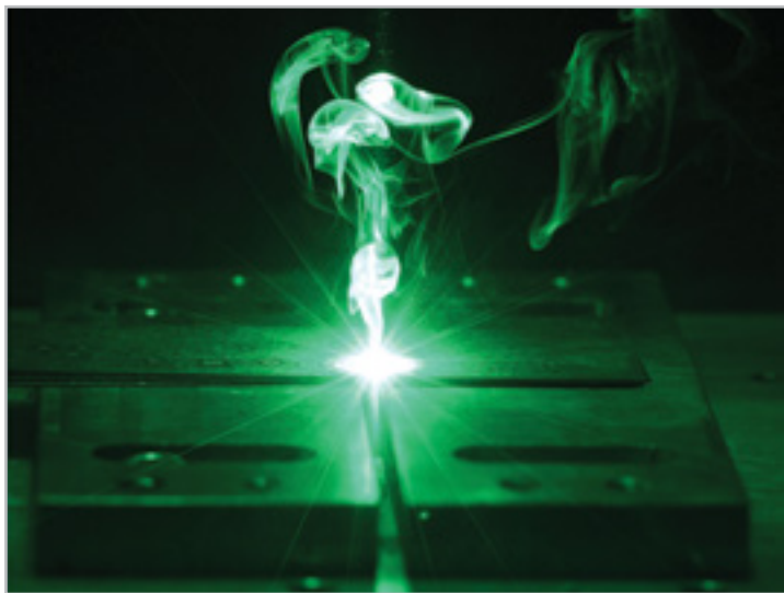
Welding with green wavelength
