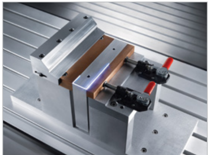
Sealing of battery housing for prismatic battery cells
