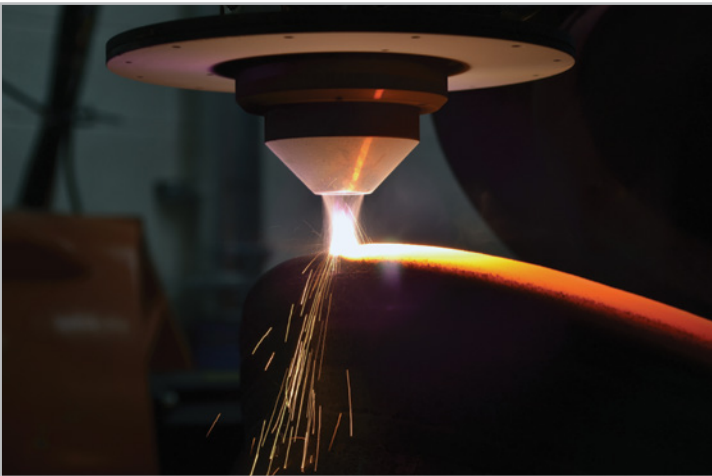
Laser Metal Deposition developed by Fraunhofer using COAX™ 8 nozzle
