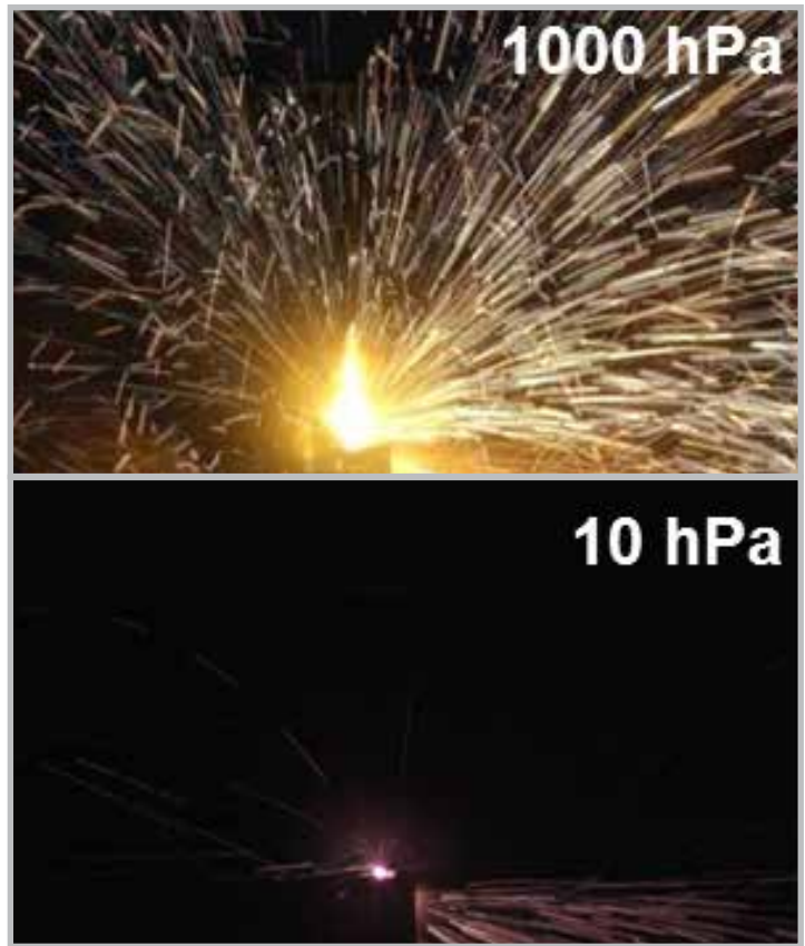
Figure 2. Process observation regarding spattering during laser beam welding
