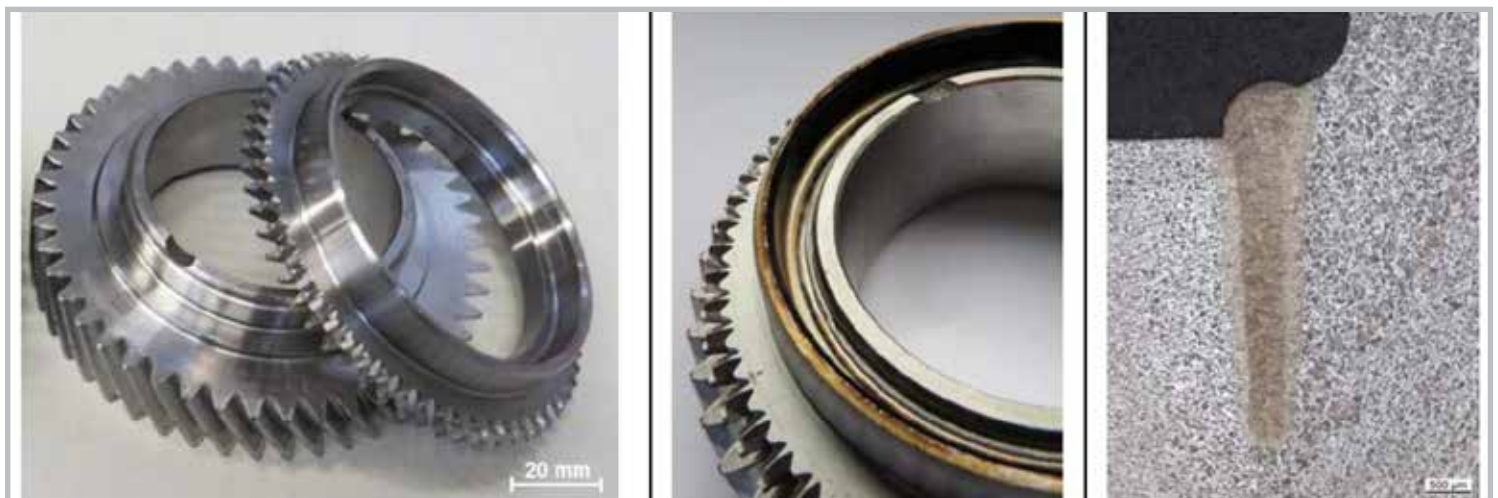
Figure 6. Typical welding application in gearbox manufacturing
