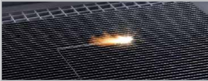
Cutting a hardened CFRP part: for materials less than four millimeters thick, the laser works two to three times faster than a water jet or milling tool and produces a higher-quality cut.
