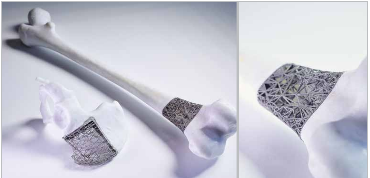
Figure of a model of a bone and pelvis with lattice type titanium implant designed and manufactured at RMIT Centre for Additive Manufacturing.
