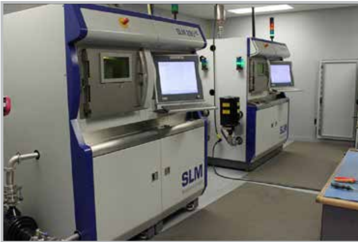
An SLM 280 HL and an SLM 280 HL “Twin-Laser” in Imperial’s additive manufacturing laboratory.
