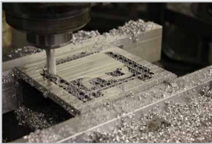
Precision machining a metal 3D printed component, part of the “Hybrid Manufacturing” approach.
