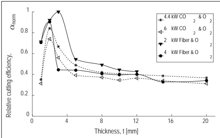
**Figure 6.2 Relative cutting efficiency results for mild steel cut with oxygen assist gas.** Note: Powers given here are the nominal maximum powers of the lasers in question. When cutting thin sections, the laser power is often automatically reduced (see notes below).
