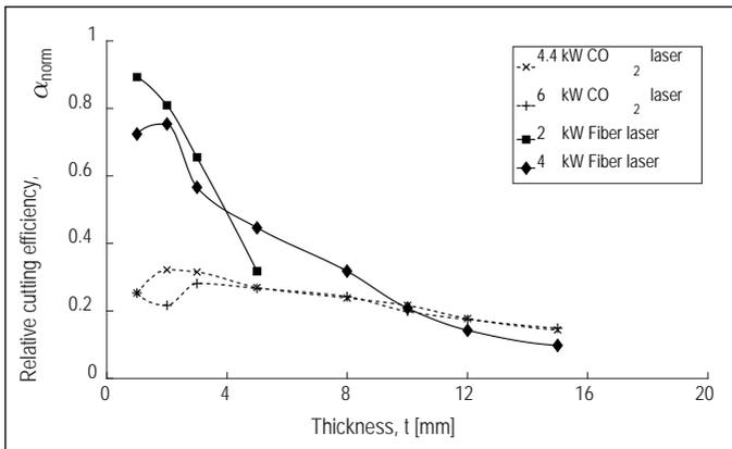
**Figure 6.1 Relative cutting efficiency results for fusion cutting stainless steel (Nitrogen cutting gas).**
