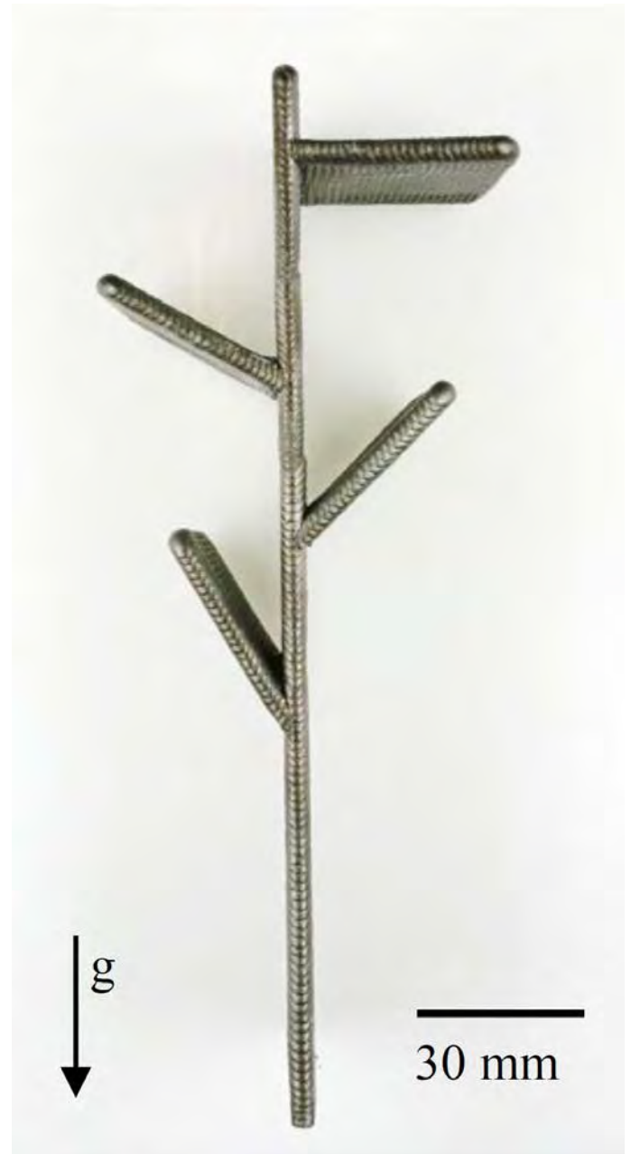
Figure 8. Manufactured overhangs with inclination angles from 30^\circ to 90^\circ .
