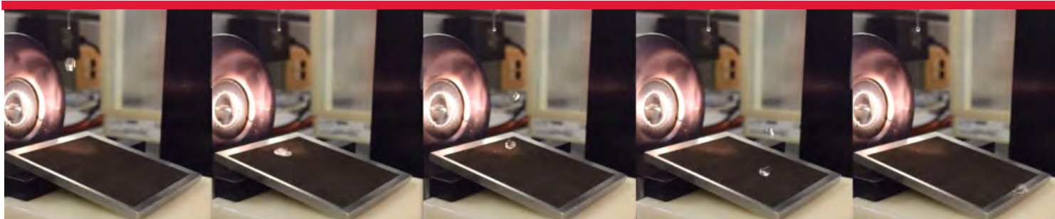
Figure 2. Superhydrophobic performance of a bouncing water droplet at \sim 5^\circ tilt.
