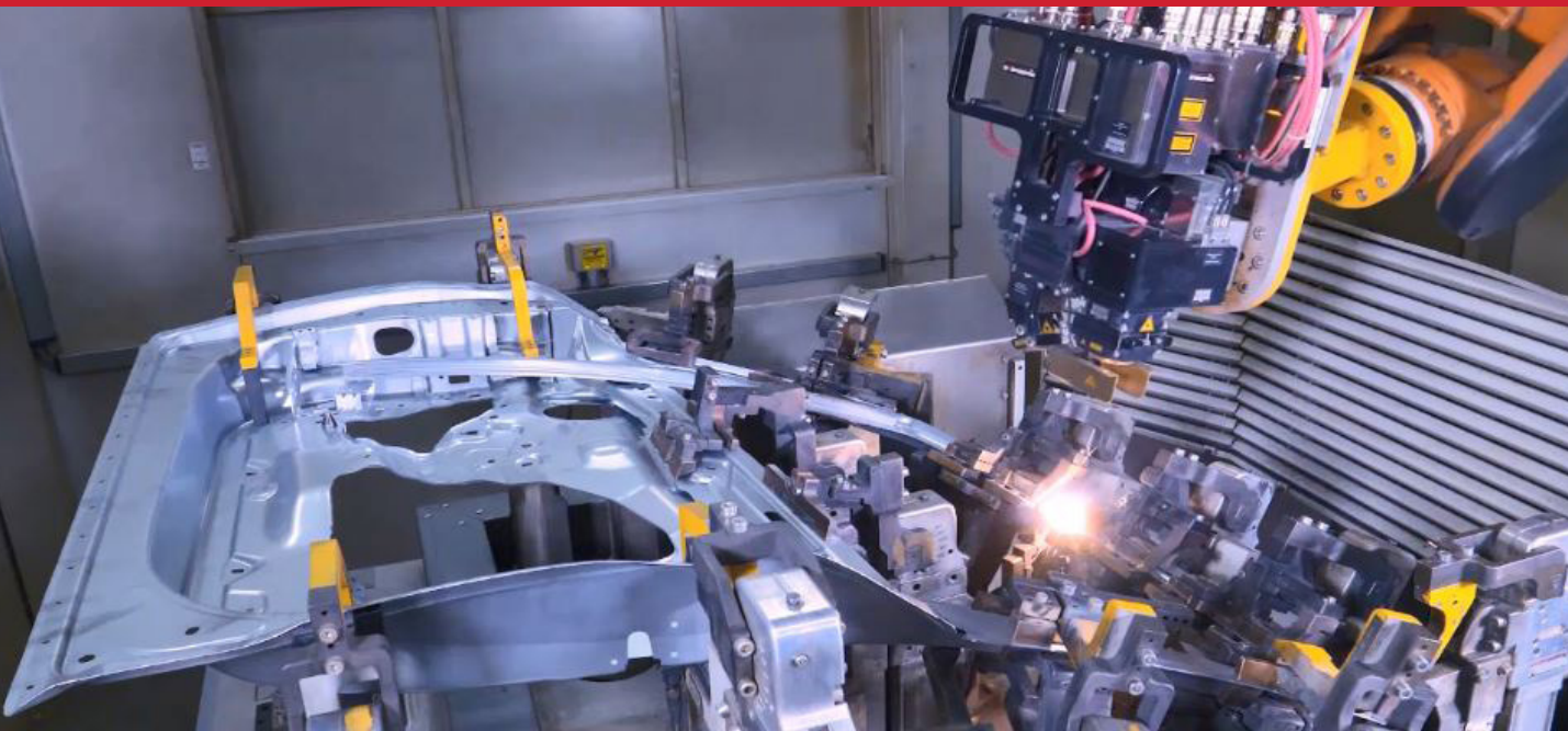
Figure 1: Production laser door welding utilizing integrated seam tracking
